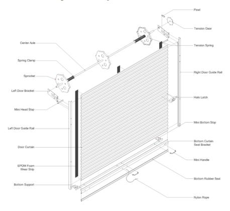
Center Axle: Made from galvanized 1-inch round tube with a 2mm inner casing for robust support.
